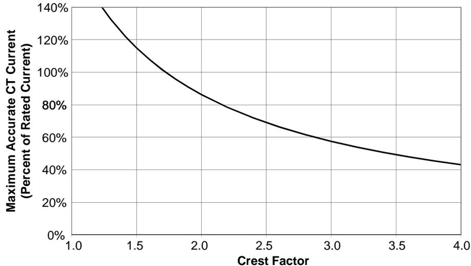
**Figure 8: Maximum CT Current vs. Crest Factor**
